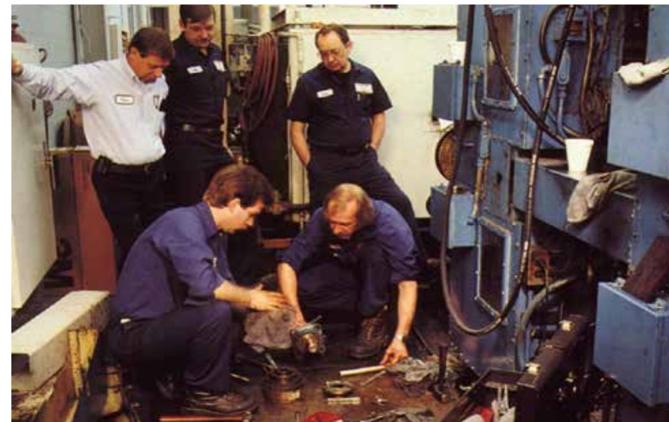
Plant shut down due to bearing failure. 80% of all bearing failures are lubrication related.
