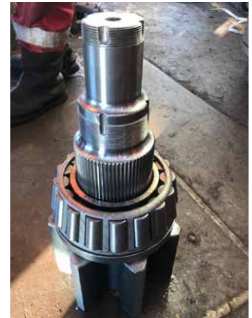
New output shaft and bearing - LeTourneau
